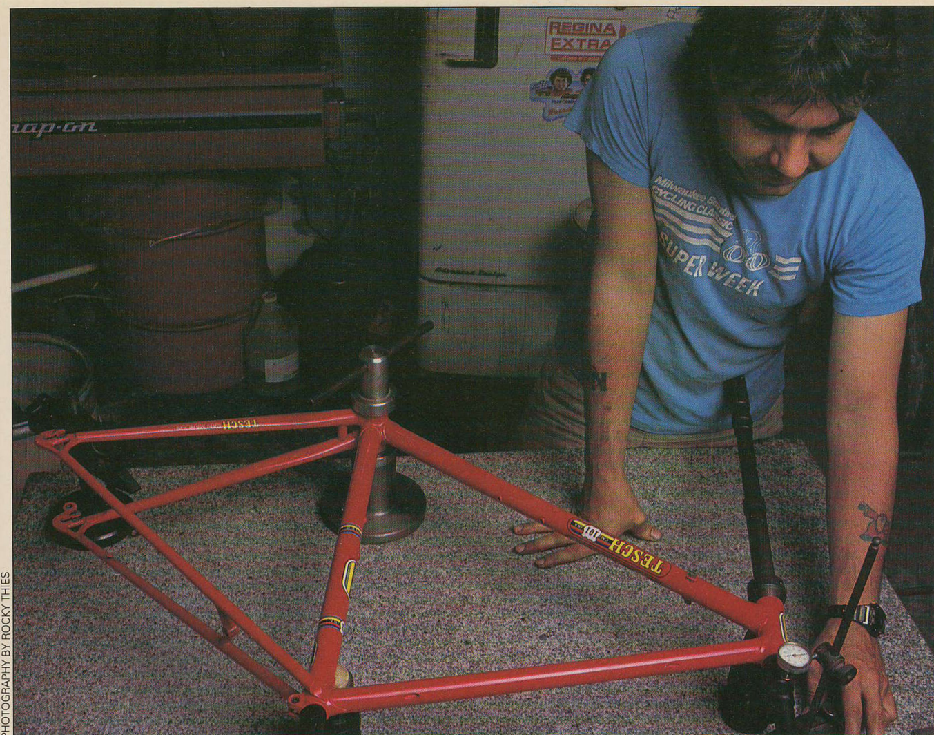
Alignment remains a labor-intensive task, but Tesch uses machines for most work. "There's no glory in mitering by hand when a lathe can do it more accurately in less time."
