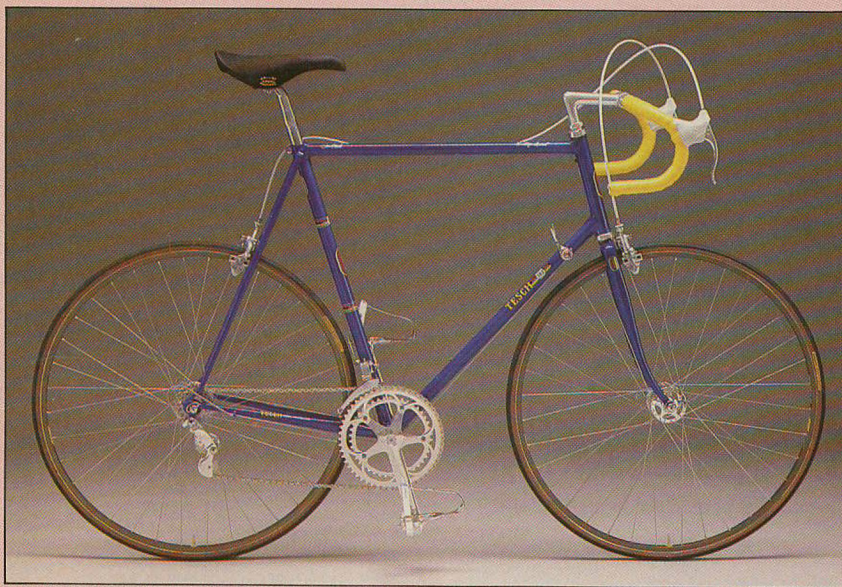
Seemingly taller than it is long, Tesch's ultra-short wheelbase 101 demonstrates how much quick handling can be built into a bike without sacrificing stability.
